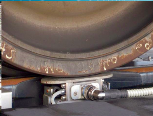
Left: Modern implementation design of an AUROPA inspection railtrack; right: Rail wheel and EMAT probe in roll-over operation
