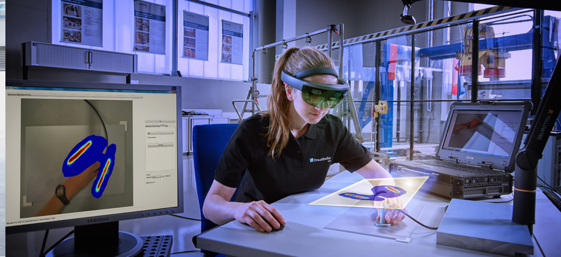
3D-SmartInspect: Augmented reality assistance system used to support manual testing of components or large surfaces
