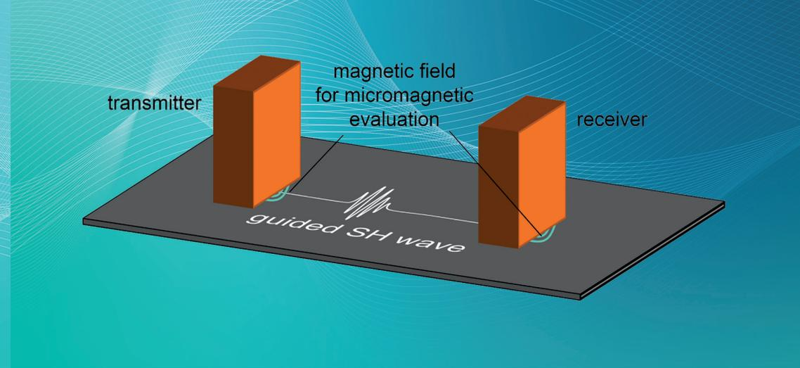
Principle of micromagnetics / ultrasonics combination
