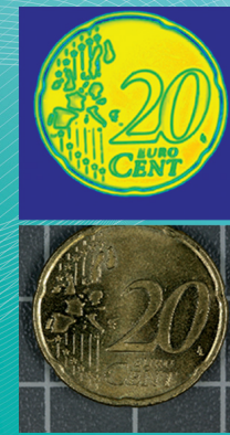
Left: Resolution of air-coupled ultrasound inspection: Coin, 1 MHz; right: Custom probe design
