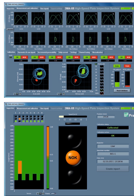
Top: extracted characteristics for the basic material (green) and hardspot (red);
