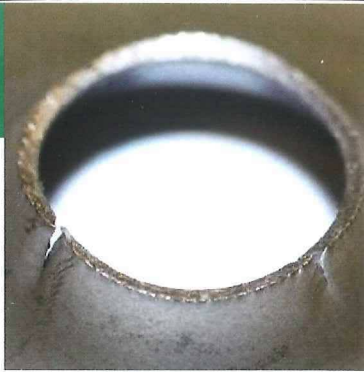
Cracks often form during collar forming.
