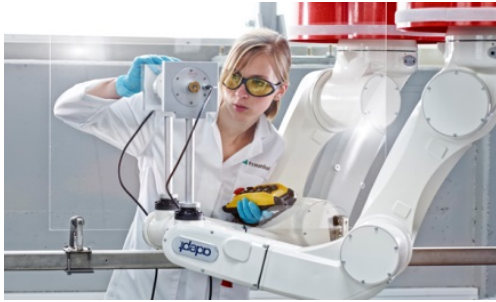
Air-coupled ultrasound: An industrial robot linked to an ultrasound inspection system scans the component. © Uwe Bellhäuser
