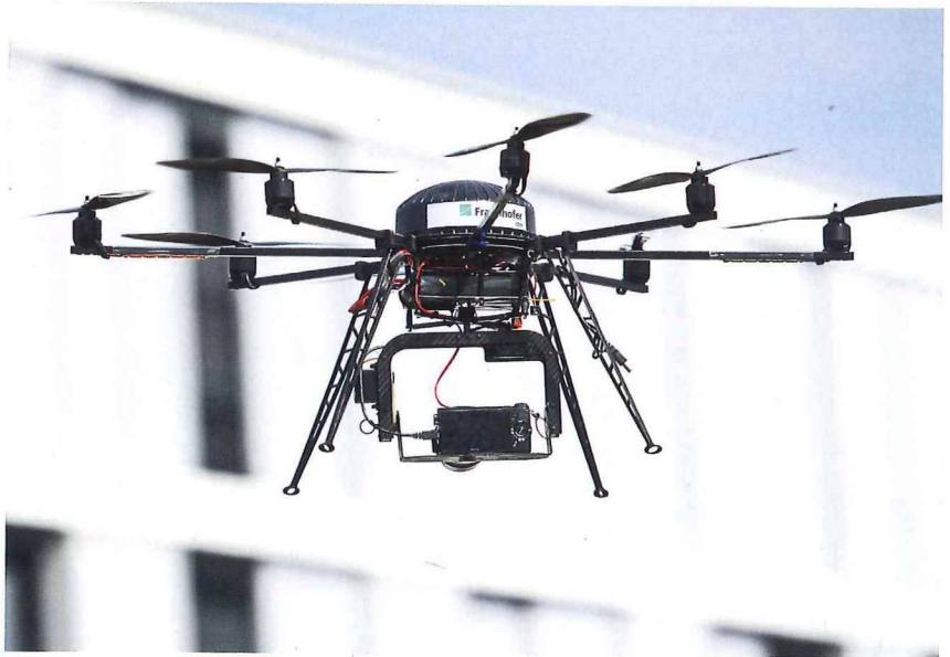
The eight rotors on the little building inspector allow it to climb more than eleven stories. Photo: Oliver Dietze
